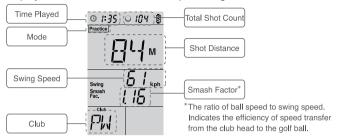
Ball Speed / Smash Factor Selection: Press and hold the + button or press the BALL/SMASH button on the remote control.
