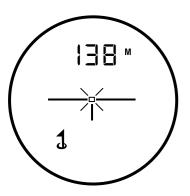
PinSeeker Indicator Aiming Reticle Active Laser Distance Displayed in Yards/Meters (To switch between Meters or Yard press and hold the Mode button)
