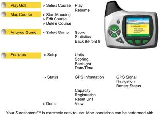
Your Sureshotgps™ is extremely easy to use. Most operations can be performed with the press of one or two keys. The soft keys change their function depending on the screen display. The function of each soft key is shown in the green bar at the bottom of the display. The menu key is used to display the main menu or exit from sub-menus.
